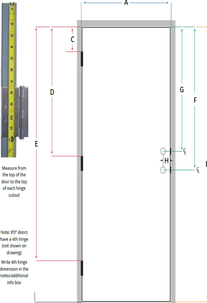
Measure from the top of the door to the top of each hinge cutout
